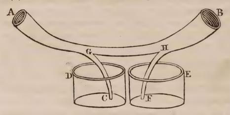
Water propelled into A, passed out at B and C, but not at F. Even if F was immersed in a coloured fluid, this ascended to H, and passed out at B with the water.
